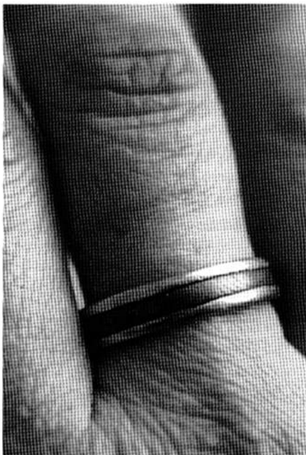
Ring (after 25 years wear): steel/22ct gold with silver lining. Steel is corroded by sweat and chemicals. Gold is changed by physical wear. The finger changes to accommodate the ring.
